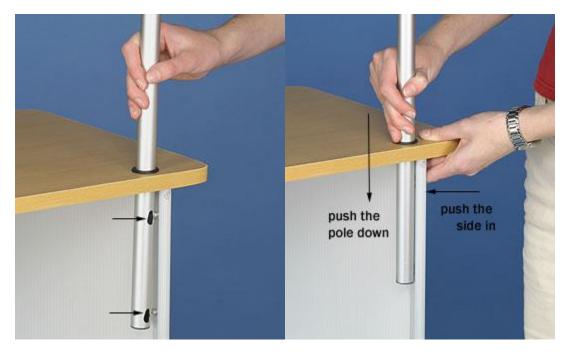
Insert each pole into the two holes in the countertop. Be sure that the Velcro<sup>®</sup> patches on the poles face front to hold the header. Line up the holes in the poles with the screws in the plastic frame. See picture left. Insert the screws into the holes, and then push down on the poles to latch them firmly in place. You may also need to push in on the plastic sides to make sure these pieces are properly connected. Once they are, your countertop will be securely attached to the frame.
